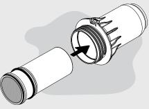
Insert the membrane module into the inflow body. 05
