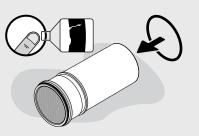
Inspect the thick black O-ring and slide into the middle 04 crevice of the module.
